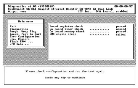
Fig. 8. Typical error message from the diagnostics program
